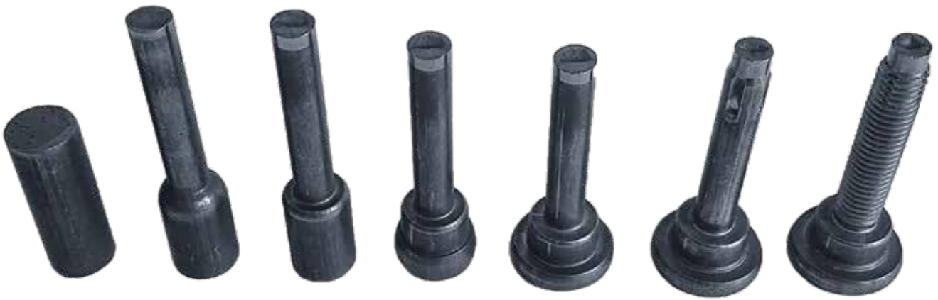
➤ Forming and rolling threads: The new CS 513 TH from Carlo Salvi can do both.
